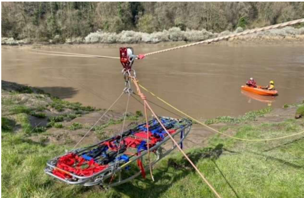
A stretcher on a 170m-long cableway across the River Wye; exercising a possible contingency plan for moving an injured caver from the mouth of Otter Hole cave to an ambulance, in April 2022
